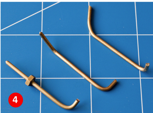
Form the metal pins to reach required shape.
